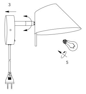
If the external flexible cable or cord of this luminaire is damaged, it shall be exclusively replaced by the manufacturer or his service agent or a similar qualified person in order to avoid a hazard.
