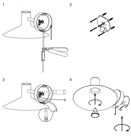
IMPORTANT:The core with green/yellow insulation must only be connected to a terminal marked with  $\stackrel{\bot}{=}$  or  $\stackrel{\blacksquare}{\bigoplus}$ .
